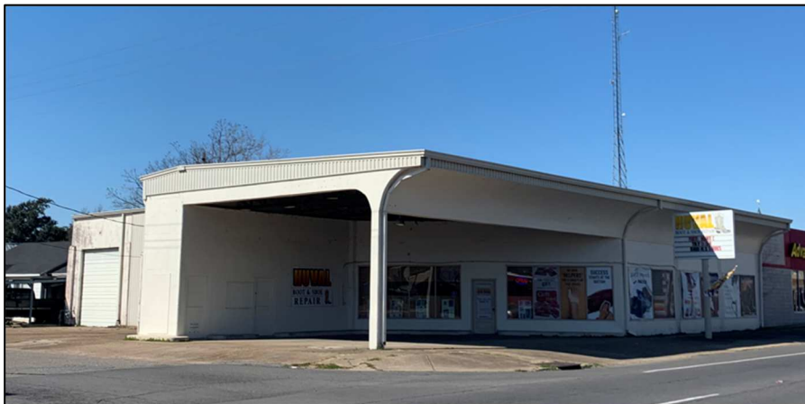
Figure 79. Huval's Boot and Shoe Repair, originally Moore-Stossell Motor Co. was constructed in 1953-54 and is constructed of a composite rice material.
